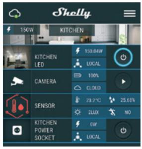
To switch the device on and off, use the **Power button**. To enter the details menu of the device, click on it's name. From there you may control the device, as well as edit its appearance and settings.
