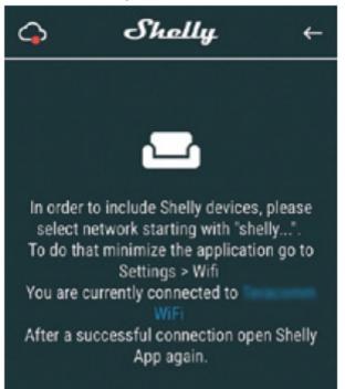
Press the home button of your iPhone/iPad/ iPod. Open Settings > WiFi and connect to the WiFi network created by Shelly, e.g. shelly1- 35FA58. If using Android your phone/tablet will automatically scan and include all new Shelly Devices in the WiFi network that you are connected to.
